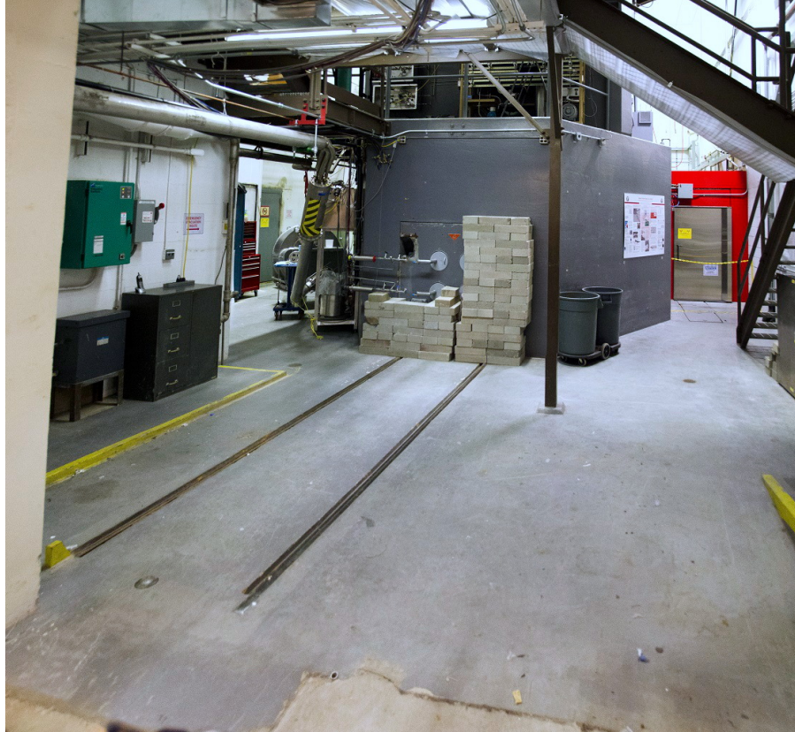
Figure 1.8: The UCN experimental area with the cryostat in its testing location to the left of the biological shield. The thermal column door is behind cinder blocks and rolls back along the tracks in the floor. The gas handling systems are just visible above the door
