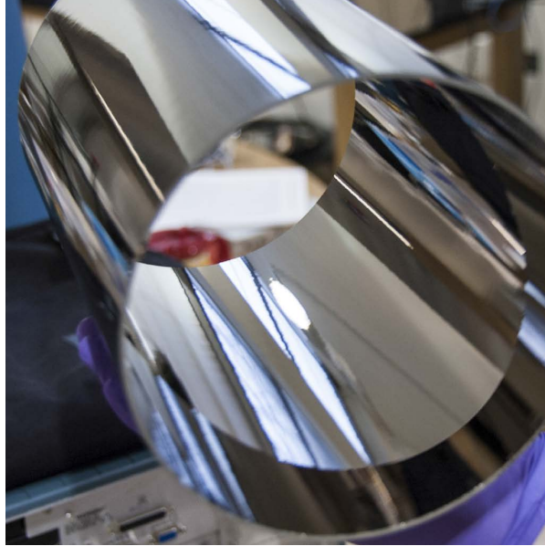
Figure 1.2: A short section of UCN guide for the Source. The 16 cm inner-diameter quartz tube is coated with nickel-58.
