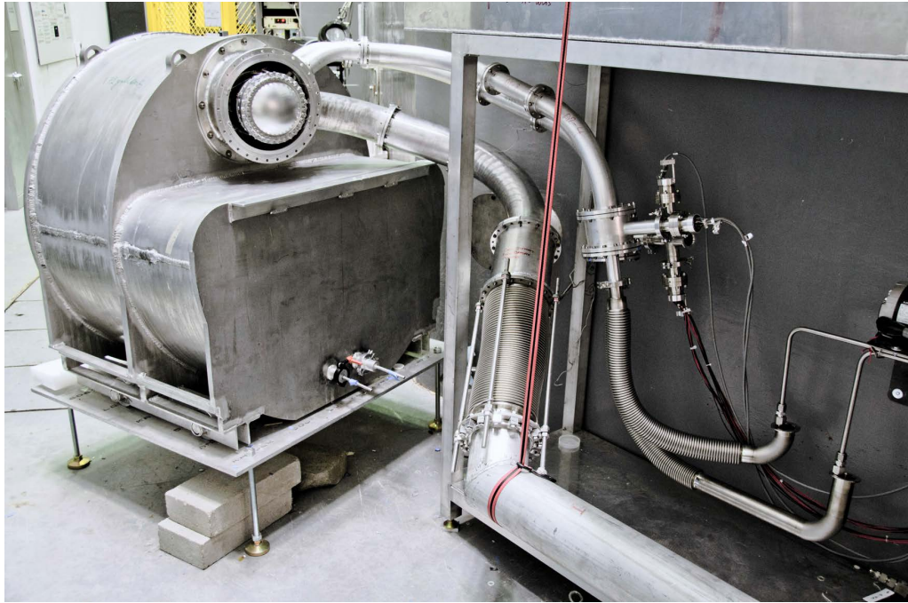
Figure 4.8: Photograph of the completed cryostat vacuum jacket from behind. Gas lines and the helium transfer tube enter from the right. The vacuum jacket is removed at the neutron guide, showing the foil window.
