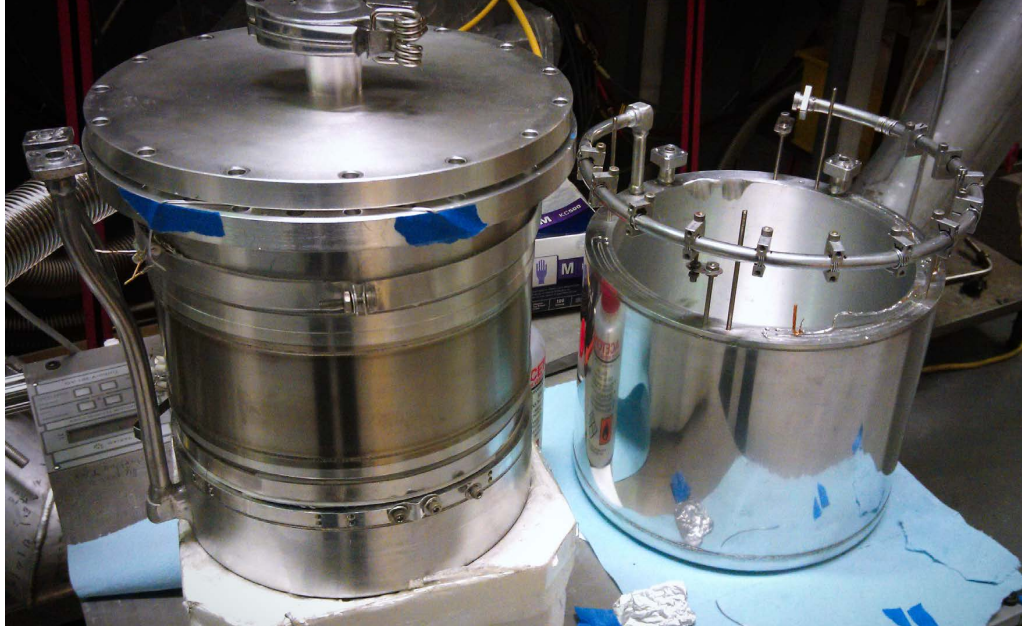
Figure 4.6: Photograph of the cryogenic containers with the capped deuterium container on the left and methane container on the right.
